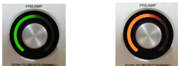
Apollo's front panel preamp knob during normal operation (left) and when a Unison plug-in is inserted in Console's PREAMP slot of Apollo's selected channel (right)
