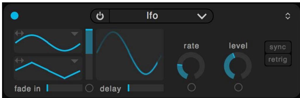
Circle 2 's LFO Module , with visual feedback. Setting rate to 1 Hz, you would see the wave repeating itself once every second.
