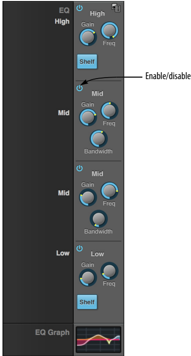
Figure 9-3: The Four-band parametric EQ module.
