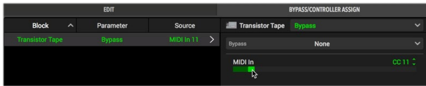
Setting the MIDI In's CC number for a bypass assignment
