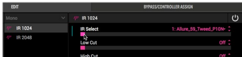
Choosing an IR by its Library (1-128) index number within the Edit tab
